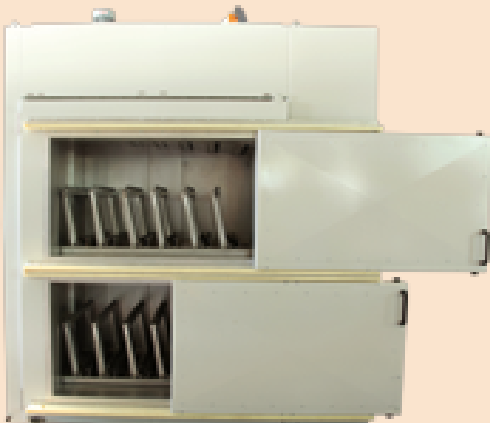
preheating furnace for model plates
