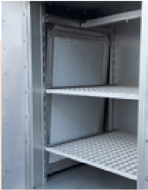
annealing furnace with HEPA cleanroom filter wall
